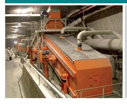
Increasing the plant capacity from 350 t/h up to 460 t/h by replacing 9 older conventional screening machines with 4 pieces BIVITEC screening machines from Binder+Co
